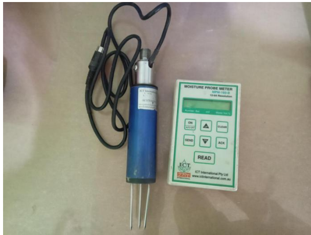
Picture1.Moisture Probe Meter (MPM) tool.
